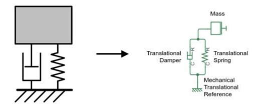
When constructing your network, it is important to include domain-specific reference blocks, such as Electrical Reference, Mechanical Translational Reference, and so on. Depending on domain, these blocks represent connection to ground, frame, or atmosphere. For more information, see "Grounding Rules".
