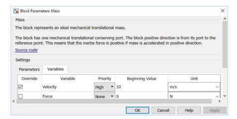
Note that the **Override** check box next to the **Velocity** variable is now selected, which means that you have overridden the default variable initialization value. This variable has high priority, therefore, the solver will try to exactly satisfy this beginning value when it computes the initial conditions to determine the simulation starting point.
